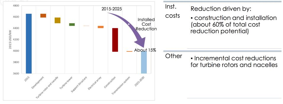
Projected installed cost reductions for offshore wind, 2015 to 2025
