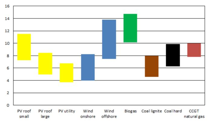
Comparison of the levelized cost of electricity for some newly built renewable and fossil-fuel based power stations in EuroCent per kWh (Germany, 2018)
