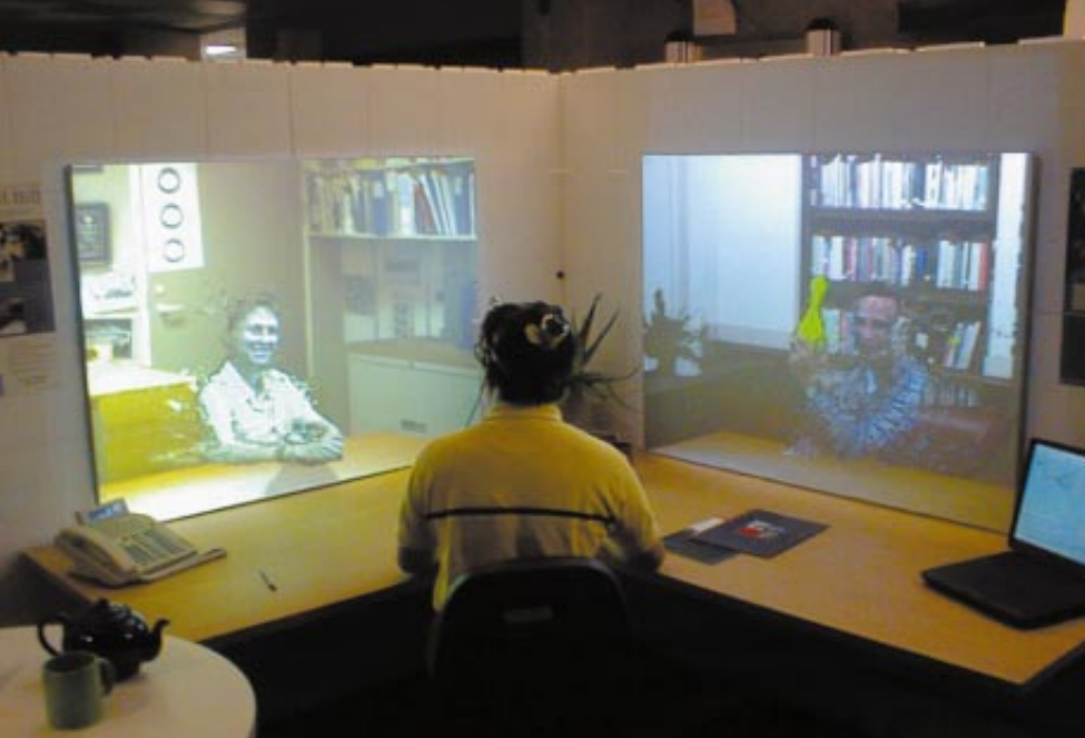
THREE USERS in different cities can share a virtual space thanks to this telecubicle.
